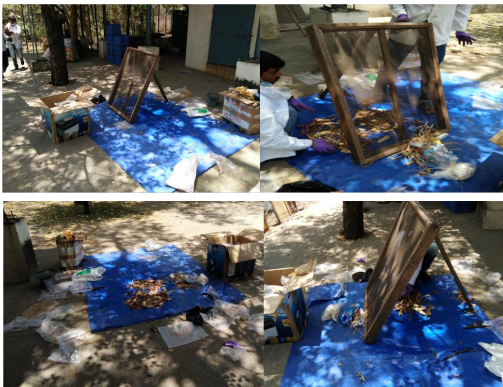
Figure 5.5 Sampling Procedure through Quartering Method
